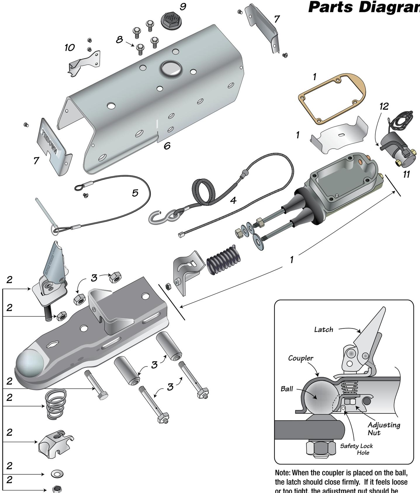
Note: When the coupler is placed on the ball, the latch should close firmly. If it feels loose or too tight, the adjustment nut should be turned to correct the fit.
