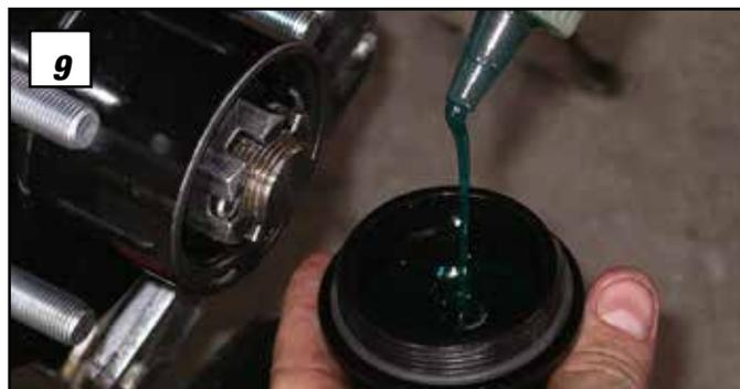
**10.** With the Turbo Lube cap filled with oil, position the cap perpendicular to the hub with the top thread of the cap lined up with the bottom thread of the threaded hub. Flip cap up 90 degrees and thread the cap onto the hub. If done correctly, no oil should spill from the cap. Torque cap to 20 to 30 ft./lbs.
