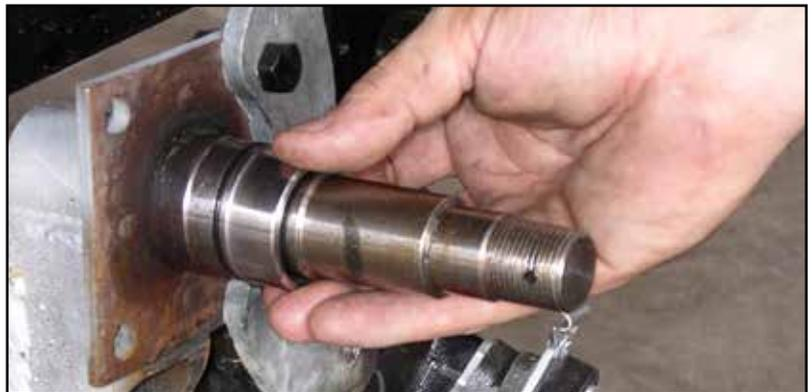
**6.** Use the wear sleeve assembly tool to properly align the wear sleeve.
