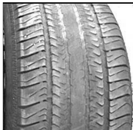
Fast Centerline Wear
