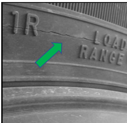
Circumferential Bead Cracking
